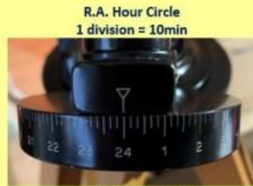
R.A. Hour Circle 1 division = 10min 0 = 24 h (=MERIDIAN) DEC axis level
