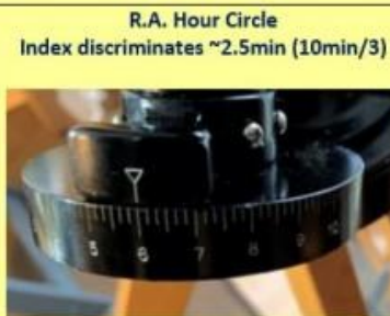
R.A. Hour Circle 1 division = 10min 0 = 24 h (=MERIDIAN) DEC axis level
