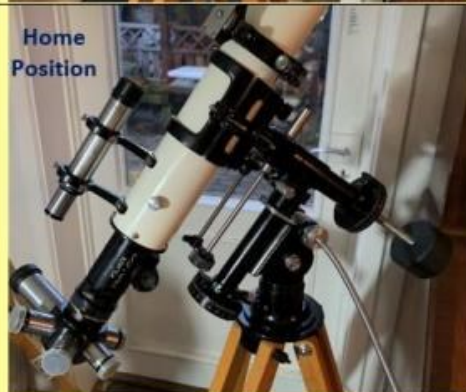
R.A. Hour Circle Index discriminates ~2.5min (10min/3) 6 h RA
