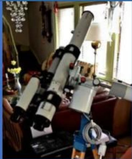
The Telemirror backend is the CZJ RACI Amici 4x EP turret, with an ATC M44 32mm EP plus Zeiss 25mm OPMI and CZJ 16 + 10mm orthos.
