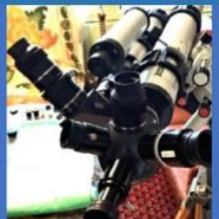
The Telemirror backend is the CZJ RACI Amici 4x EP turret, with an ATC M44 32mm EP plus Zeiss 25mm OPMI and CZJ 16 + 10mm orthos.
