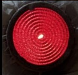
Flat1: <10 λ precision Van Keuren Co. mirror Focus (Null)
