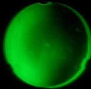
Flat1: <10 λ precision Van Keuren Co. mirror Focus (Null)
